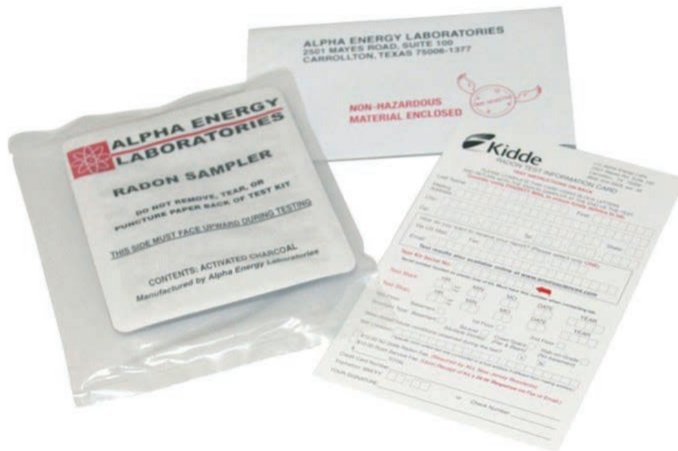
The HCN Division of Environmental Health uses Radon Test-Kits, like the one pictured, to test Tribal Member's Homes
